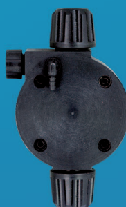
PVC pump head for high flow rate ( 20 lt/h up to 50 lt/h) complete with ball injection valves (ceramic balls) FPM or EPDM seals
